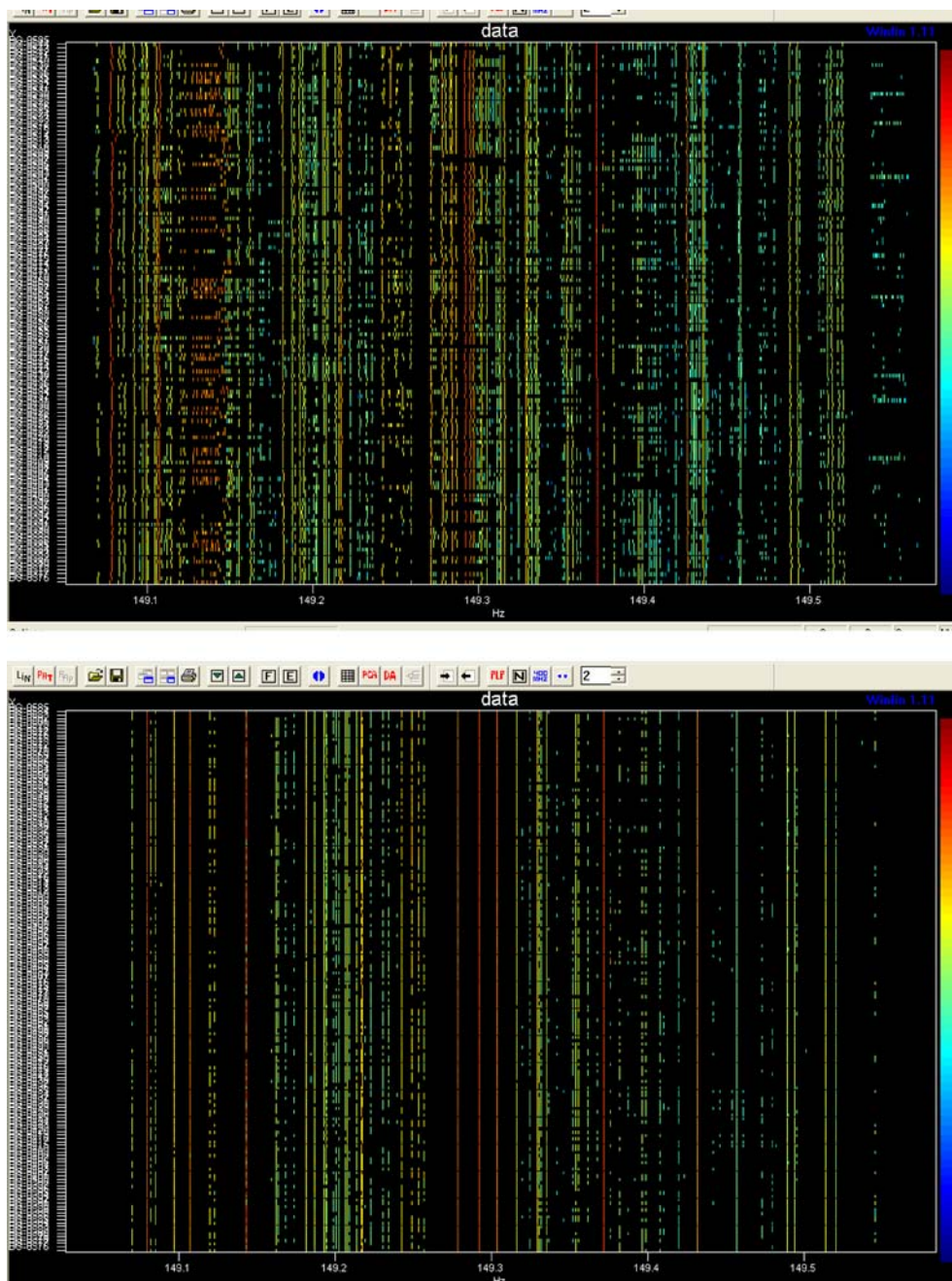
Fig. 5 Plot of a series of samples analyzed by GC-MS before ( upper figure ) and after ( lower figure ) alignment of the retention time and application of an appropriate threshold
